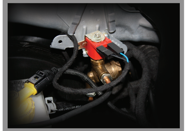
Gaz kesicinin araca yerleşimi Mounting the gas cutter to the vehicle.
